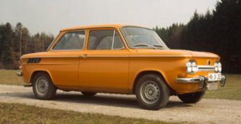
An improved NSU TT hit the market in 1967. Its 1200 cc engine producing 65 hp made it one of the fastest in its class as standard. The round dials on the dashboard were now combined on an aluminium panel.
