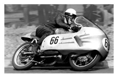
For the 1955 season, DKW extensively modified the 350 cc racing motorbike that was previously used and made it stable. In August, the engineers in Ingolstadt presented a single-cylinder racing machine with a 116 cc engine that was derived from the 350 cc bike, and this was to compete in the 125 cc class.
