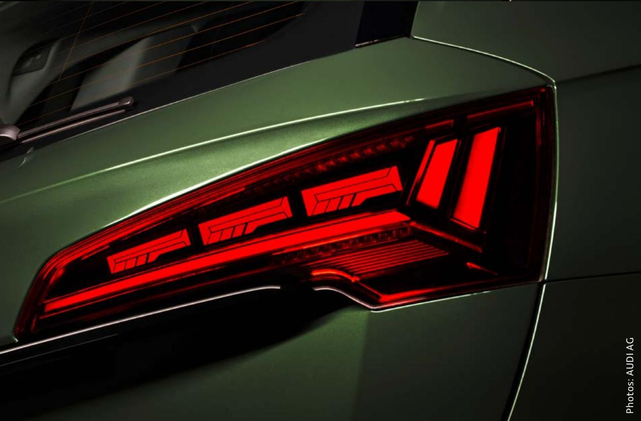
An Audi Q5 rear light has three panels, each incorporating six OLED segments. These can now be activated as needed, and their brightness adjusted infinitely. The optional proximity detection by activation of all OLED segments can be seen at the bottom.
