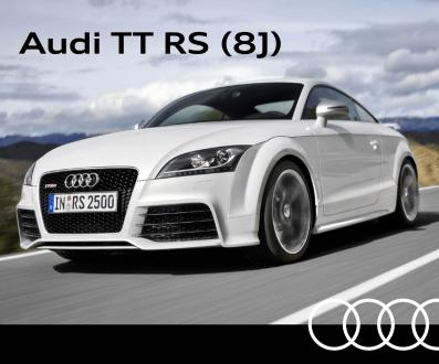
The TT RS is the most powerful and fastest sports variant in the Audi TT's second generation. It has a transverse-mounted turbocharged 2.5 liter five-cylinder engine under the hood. Launch: **2009**
