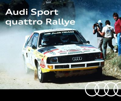
The wheelbase was shortened by 32 centimeters (12.5 inches) as compared with the "Ur-quattro." The Sport quattro is a light, compact powerhouse so it can meet the homologation requirements for group B rally cars.
