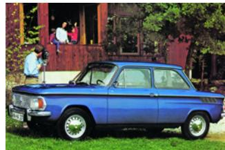
The inspiration to build this fast compact car came from NSU’s Head of PR, Artur Westrup. The initial version of the NSU TT, powered by a 55 hp engine, was characterized by front disc brakes, dual carburetors, a tachometer, twin headlights, and a steering wheel with two perforated aluminum spokes.
