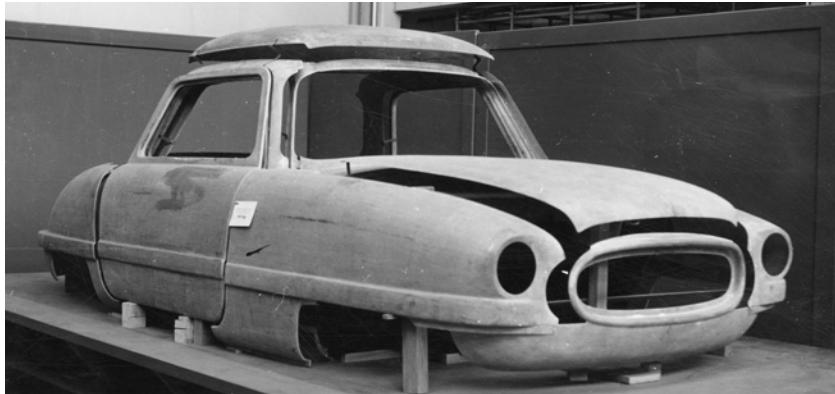
In addition to the technical uncertainties of mass-producing plastic bodies – an area with no comparable references at the time – the departure of the two key figures, Eberan-Eberhorst and Kurt Schwenk, in September 1956 led to the termination of all work on DKW plastic cars. Nevertheless, foundational research on plastic body components continued at the Düsseldorf plant until it was sold to Daimler-Benz AG in 1962.
