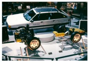
A 181 kg nickel-cadmium battery that had a capacity of 8.6 kWh and could be charged rapidly delivered power for the electric drive and demonstrated the feasibility of hybrid vehicles that can travel without producing any exhaust emissions on short journeys. To switch from one operating mode to the other, the car had to stop and be switched over to electric drive with the combustion engine switched off.
