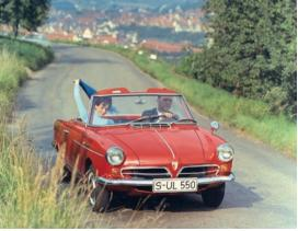
The Wankel Spider was the world's first mass-produced car to be powered by a single-disc rotary piston engine which had a volume of 497 cc and produced 50 hp. Since the beginning of the 1950s, NSU had worked with Felix Wankel to produce a completely new engine concept. With the NSU Wankel Spider, the engineers in Neckarsulm demonstrated that this engine did not just work on test benches.
