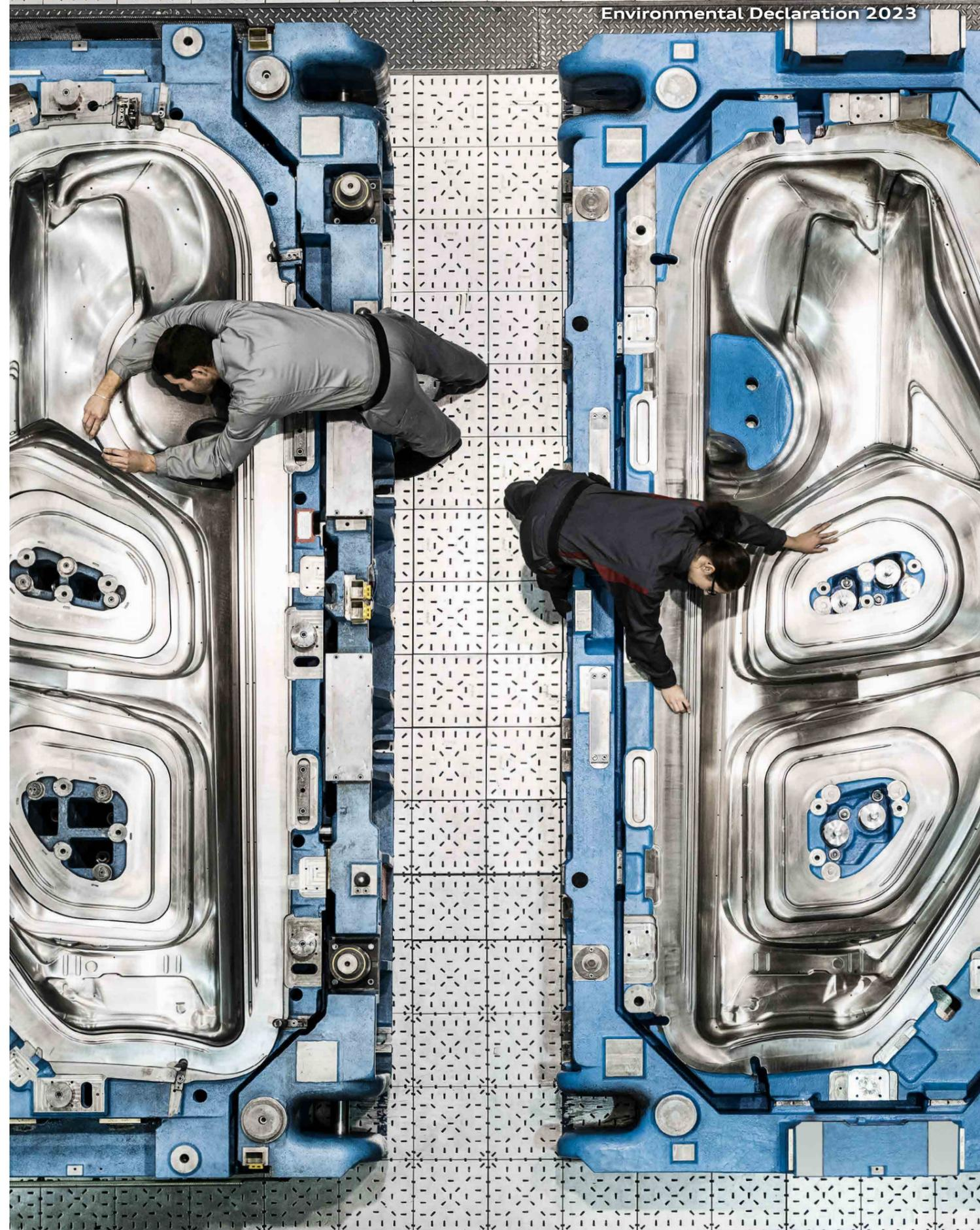
Press Shop - unfolded tool for side wall frame
