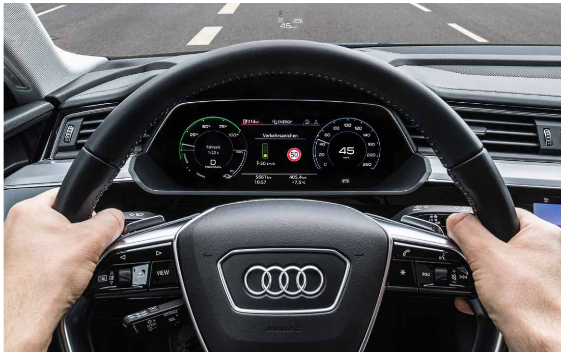
In the cockpit, drivers see not only the current speed limit but also how fast they must drive to reach the green light.
