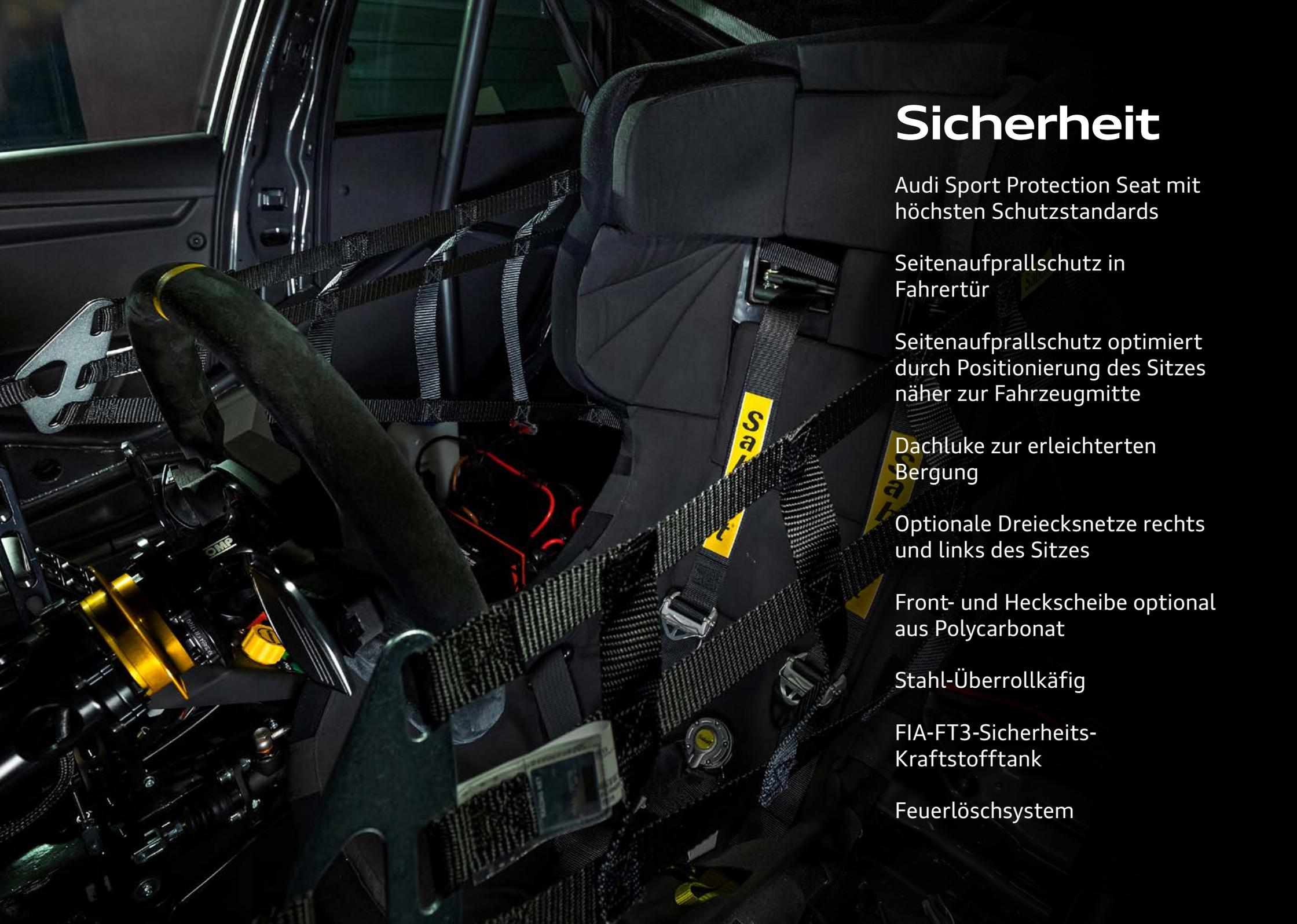
The image shows the interior of a race car, focusing on the driver's seat. The seat is a dark grey racing seat with a complex harness system consisting of multiple black straps with silver buckles. A roll-over protection structure (ROPS) is visible, made of metal bars. The steering wheel is partially visible on the left, featuring a yellow OMP logo. The overall lighting is dim, highlighting the textures of the seat and the metallic components.
