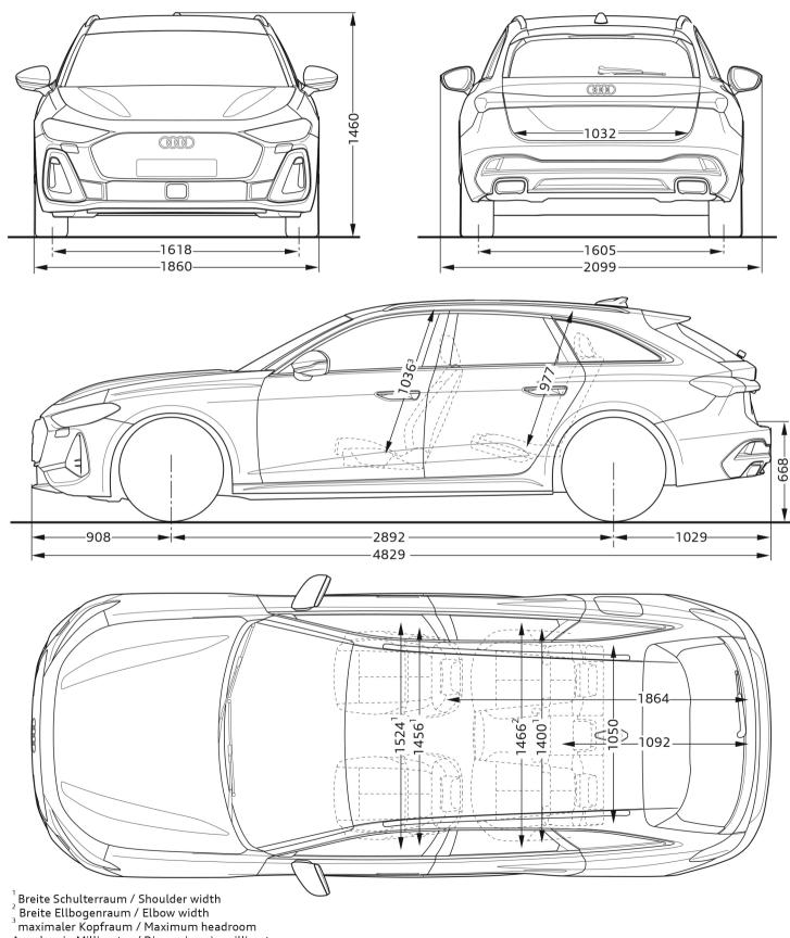
Angaben in Millimeter / Dimensions in millimeters
